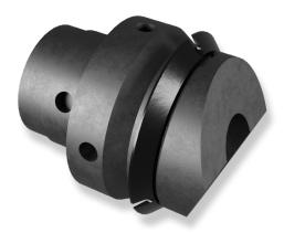
Whether your perforating guns misfire, you need to pump guns down for stage one, or you simply want to log the well without using a gauge ring, the PurpleSeal™ Pump Down Nose is up for the challenge. With an entirely composite construction, it can be released downhole if desired. The pumpdown fin feature drastically improves the pumpdown efficiency by creating more surface area for the water to pump on; it effectively pulls your assembly downhole.
