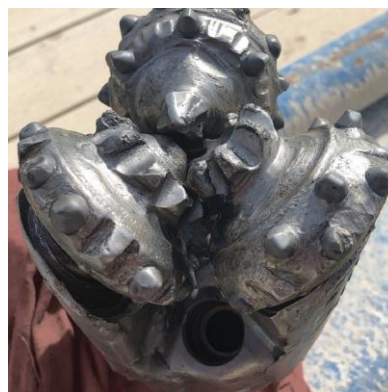
Taurex Bore Haug tri-cone bit after drilling out 104 composite frac plugs. Normal insert wear, rollers intact.
