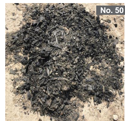
Drill-out debris from PurpleSeal plug No. 50.
